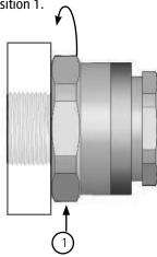
2. If it is necessary to tighten the components of the insulated adaptor, then spanners should be used at positions 1 and 2. The max torque to be applied is shown on the back page.
