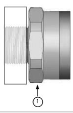
2. Tighten the cable gland into the insulated adaptors using spanners at positions 1 and 2. The max torque to be applied is shown on the back page.
